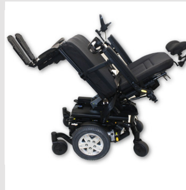
Mid-wheel drive power wheelchair using power tilt
